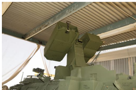
Jun. 23, 2017 | Marine Corps Logistics Base Barstow, Calif. - The Modified Target Acquisition, MTAS, turret swivels through its paces as the last of the testing is performed on the newest rocket launcher for the Light Armored Vehicle Anti-Tank vehicles, at Production Plant Barstow, Marine Depot Maintenance Command, aboard the Yermo Annex of Marine Corps Logistics Base Barstow, Calif., June 15. Crews from production plants Barstow and Albany, Ga., are training at PPB to learn how to install the new MTAS turrets. Photo By: Keith Hayes
